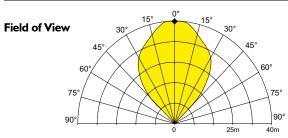
To meet the requirements of EN54:10 dause 5.4, where the ratio of the response points. Dmax: Dmin should not exceed 1.41, the horizontal and vertical viewing angles max should not exceed  $\pm 30^{\circ}$ .
