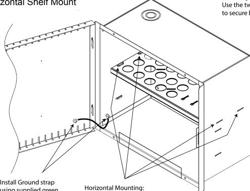
Install Ground strap using supplied green wire and 8-32 nuts.
