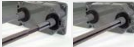
INSERT ADAPTOR, INTERCONNECT TUBES & TURN TOWARD AIRFLOW
