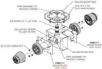
\*Includes 2 mounting plates and 1 blank mounting cover plate. See over for mounting holes diagram
