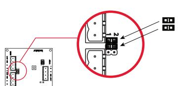
The Isolator EOL jumpers may need to be added if the riser side of the isolator is the last device of the branch. Jumpers must be installed on pins 1-2 and 3-4 as shown to add the EOL.
